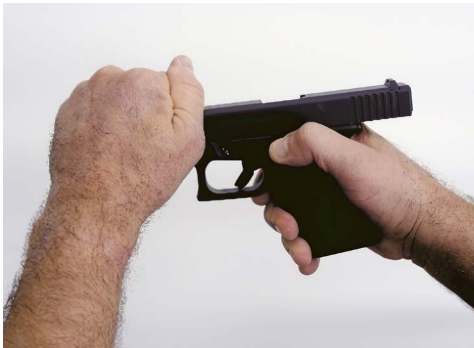
Fig. 9. Slide locked to the rear during firearm inspection.
